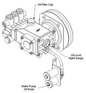
2. After the first **50 hours** of operation, change the crankcase oil with CAT Pump Crankcase Oil, (Part # 13-000). Change the crankcase oil every **500 hours** thereafter.
